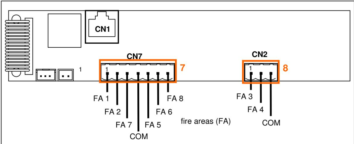
8 Connect to control outputs for faults in the fire areas 1, 2, 5 -8. For details refer to table “CN7 FA connections”
