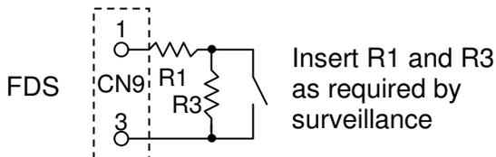
When control output is monitored and activation by breaking a contact
