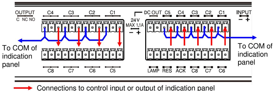
→ Connections to control input or output of indication panel
